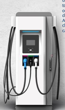
The Piccoli charger eFelx DC fast charging station is a dual DC outlets (CHAdeMO and CCS) 60 to 120kW (up to 160kW) fast charger with an optional Type-2 AC output up to 22kW that can be configured to meet different charging needs of both European and North American customers. It supports all three connectors charging simultaneously and balancer reel for advanced cable management.
